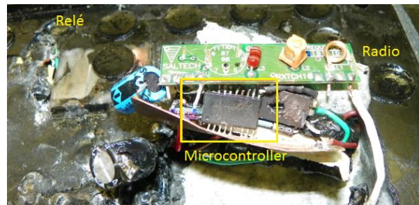
Figure 7 – printed circuit board and wire-up circuit removed from the epoxy resin
