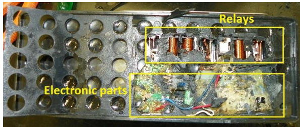
Figure 4 – The verification switch and abnormal electronic devices hidden under the epoxy resin [15]
