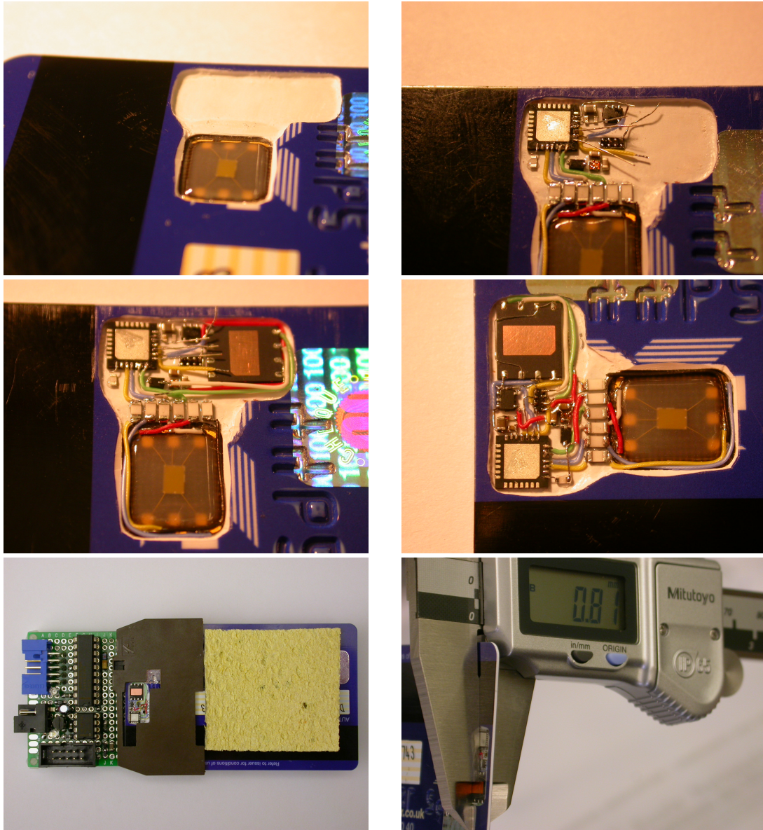
Figure 3. Passive monitoring card containing real EMV chip, with monitoring microcontroller and flash storage
