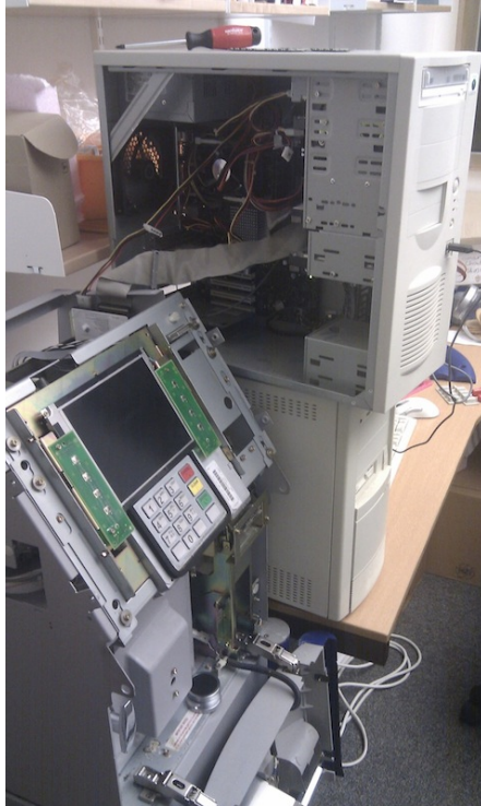
(a) Extracting disk image from NCR ATM
