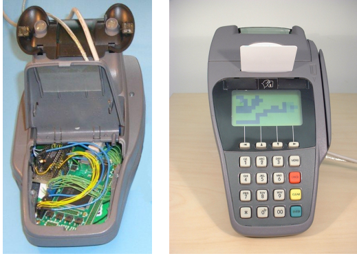
Figure 6. Modified Chip and PIN terminal, playing Tetris
