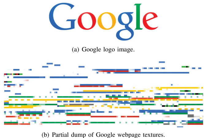
Figure 1. Google logo and partial dump of Google webpage textures extracted from the Chromium web browser with an NVIDIA GPU.
