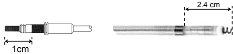
Figure 7. Illustration of the connector and tip of typical active fixation corkscrew bipolar pacemaker leads. The central cathode connector is extended further than the external anode and the cathode tip protrudes further than the anode ring.
