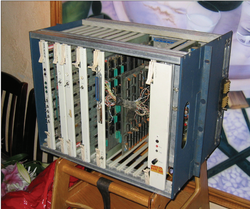
Figure 2. Northern Telecom SL-10 packet switch, the foundation of the Datapac network.
