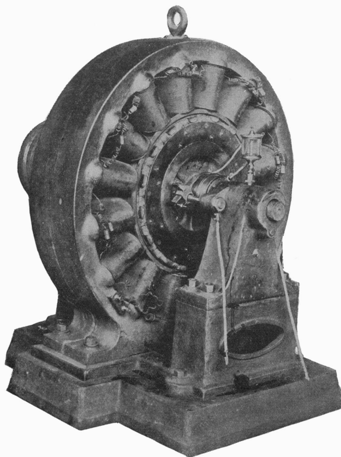
A 16-pole a-c generator installed in a plant of the Brush Electric Light Company, Buffalo, N. Y., on November 30, 1886. The design was the work of Stanley, Shallenberger, and Schmid
