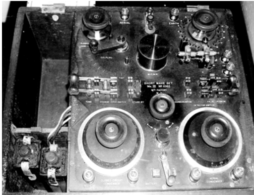
Fig. 6 1915 short-wave crystal receiver for use in trench warfare
