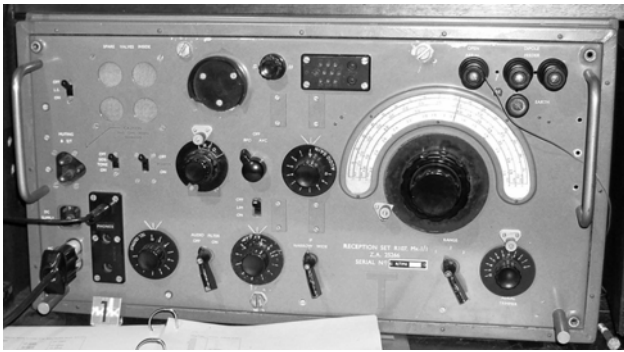
Fig. 3 R107 Communications Receiver, 1.2–17.5 MHz
