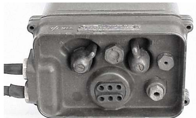
Fig. 13 Control panel of WS 88
