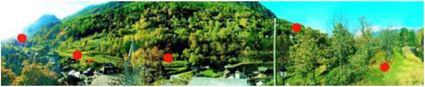
Fig. 3. Panorama from the “Pierre Bergère” (Shepherdess Stone) showing the places reached by the wireless transmissions, indicated by red dots. From right to left: Les Maraïches (5-200 m), Le Creté du Serré (~400 m), Ladray (~500 m), La Combaz (~400 m), and Les Marécottes (~1600 m).
