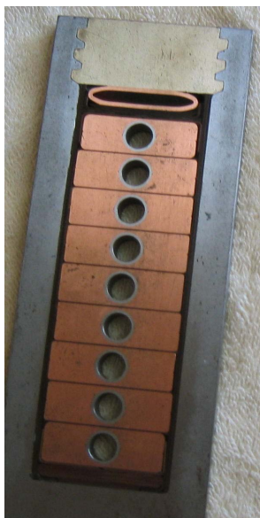
Figure 4. Cross section of water-cooled turbo-generator rotor slot with stainless steel cooling tubes.
