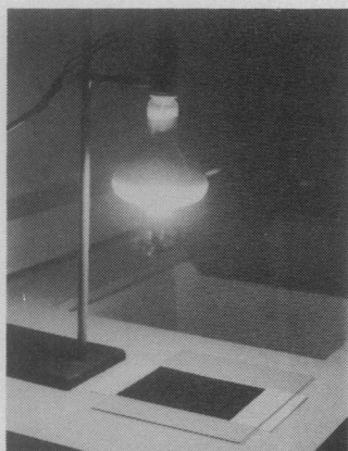
Fig. 5. Exposing Blue Poly film with sunlamp
