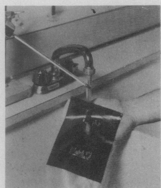
Fig. 6. Washing out Blue Poly after exposure
