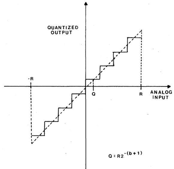
Fig. 2. Quantization using an ideal 3-bit A/D converter ( $b = 2$ ) set to produce roundoff errors for analog input data in the range  $-R$  to  $+R$ .
