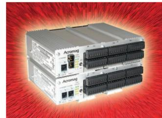
The ES2113 interfaces with any mix of up to 96 discrete input and/or output signals. Inputs and outputs are connected in tandem with each other for easy "loop-back" monitoring of the output to increase system reliability. Selectable internal or external excitation on each 16-channel port simplifies wiring and increases flexibility for five–28 Vdc logic.
