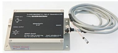
The Hall probe chip incorporates horizontal and vertical Hall elements, analog electronics, and a synchronization circuit. Current spinning in the Hall devices cancels offset, 1/f noise, and the planar Hall voltage. The external analogue electronic module of the transducer cancels the residual offset and compensates the temperature dependence and non-linearity of the Hall voltages.
