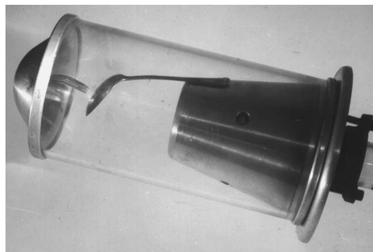
Fig. 6. Fork and spoon X-ray tube.
