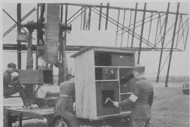
Fig. 10—Detailed view of range-finding equipment located in rear of azimuth antenna. May, 1937, tests.
