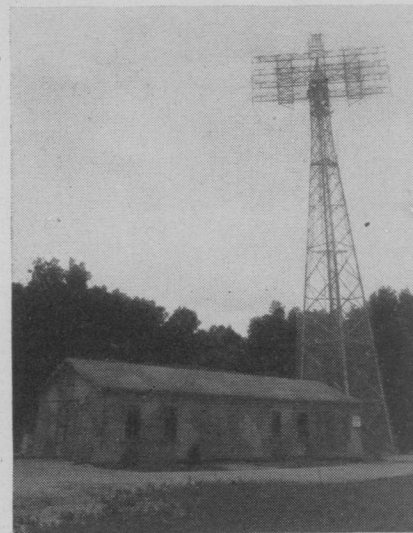
Fig. 31—Radio set SCR-271-D at the Evans Signal Laboratory, showing shelter for components and operating personnel, 100-foot tower, and antenna modified for plan-position-indicator display. Identification, friend, foe (IFF) antenna is shown at top center on radar antenna.
