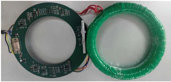
FIGURE 9. The image of the self-oscillating fluxgate sensor.
