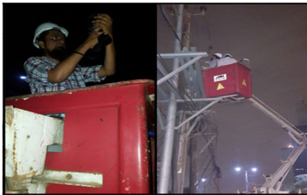
FIGURE 5. Data acquisition using thermal imaging camera.
