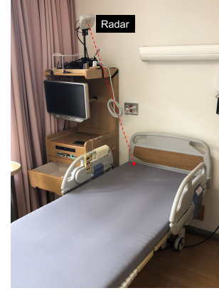
Fig. 2. Measurement setup with millimeter-wave array radar system in a hospital room.
