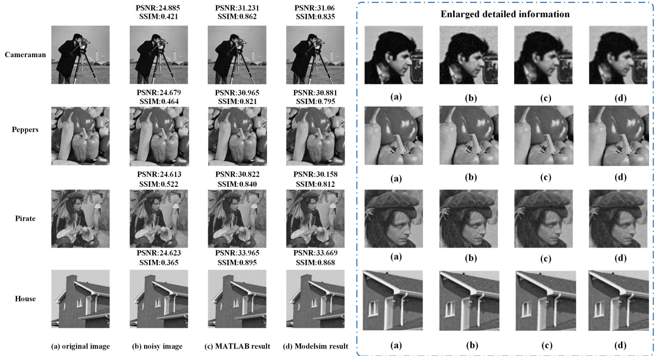
FIGURE 8. Comparison of the MATLAB results and the ModelSim results ( \sigma_n = 15 ; \sigma_r = 45 ).
