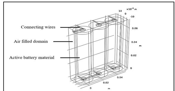
**FIGURE 1. Geometry modelling of the battery module [23].**
