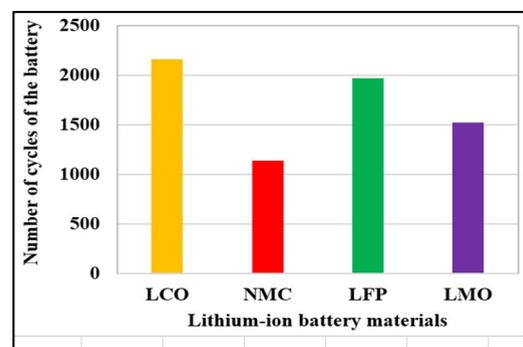
FIGURE 15. Number of cycles of the battery.
