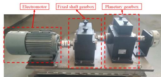
FIGURE 17. Laboratory planetary gearbox fault data test rig.
