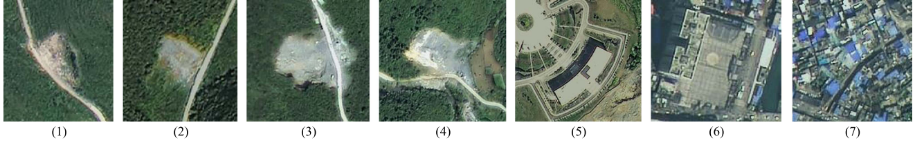
Fig. 10. Exemplified images of the Bijie Landslide dataset [13], where (1)–(4) are landslide images, and (5)–(7) are nonlandslide images.
