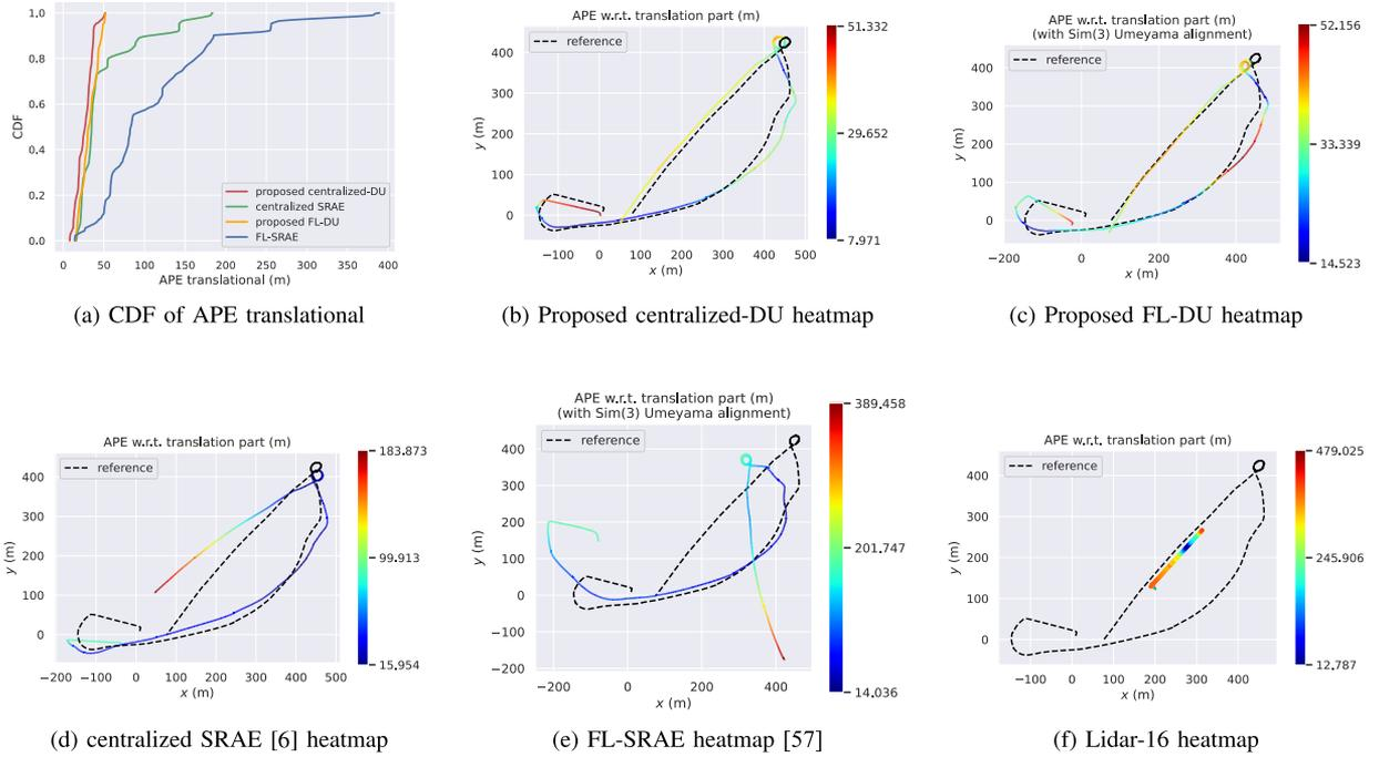
Fig. 7. CDF and heatmaps for the centralized DU method, the proposed FL-DU framework using the DU model derived from the 50-th communication round, the 16-channel Lidar and the method SRAE [6] using as reference trajectory the path derived from the lidar with 64 channels regarding the first path with the 6000 scans. Note that in the CDF plot, the 16-channel Lidar was excluded due to its insufficiency to yield satisfactory comparative results.
