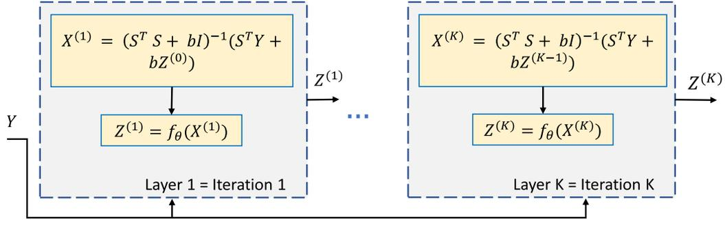
Fig. 2. Proposed Deep unrolling model. In particular, a small number of iterations, say K, of the local HQS solver in (11) are unrolled and treated as a deep learning architecture. Each iteration of the iterative solver is considered a unique layer of the proposed model, resulting in a K-layer deep learning architecture.
