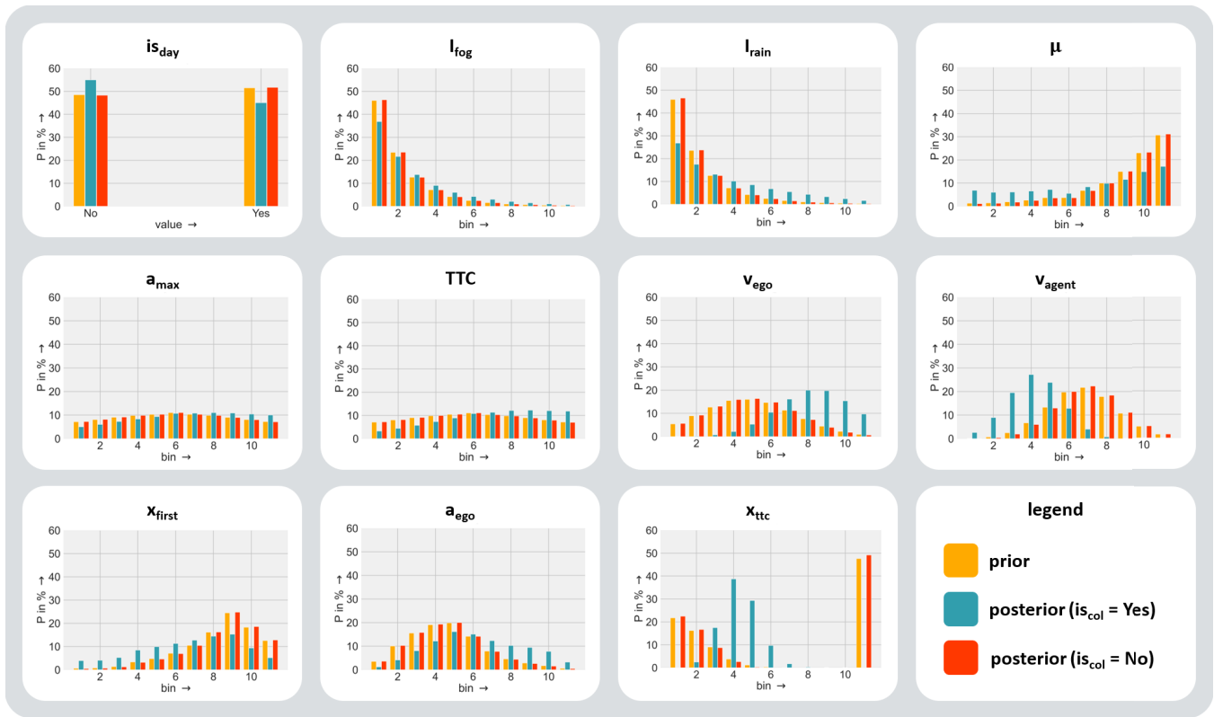
Fig. 9. Probability distributions given a collision (blue), no collision (red), or no condition (yellow).
