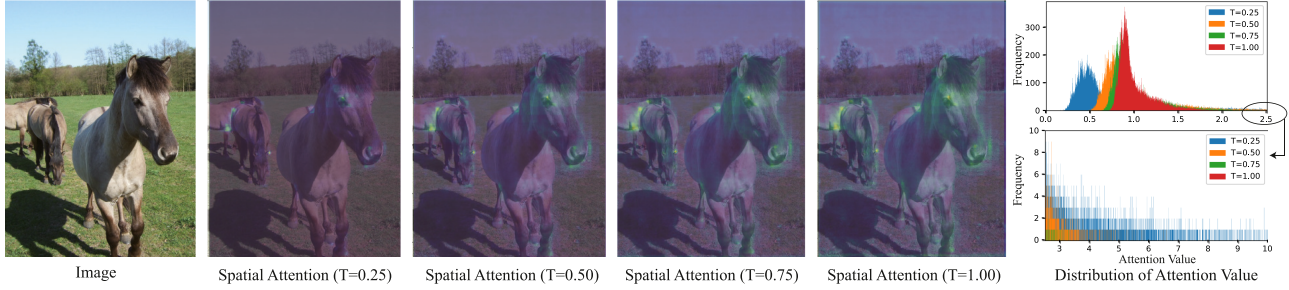
Fig. 4. Visualization and distribution of the spatial attention with different T (temperatures) in attention-guided knowledge distillation. With a smaller T , the pixels of high and low attention values are emphasized and suppressed more in knowledge distillation, respectively.
