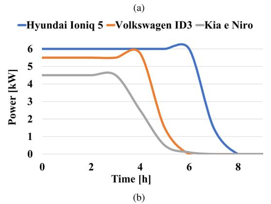
Fig. 4. Charging characteristics of EV batteries. (a) Fast charging. (b) Slow charging.
