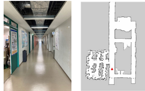
FIGURE 3. Mapping result by using SLAM.
