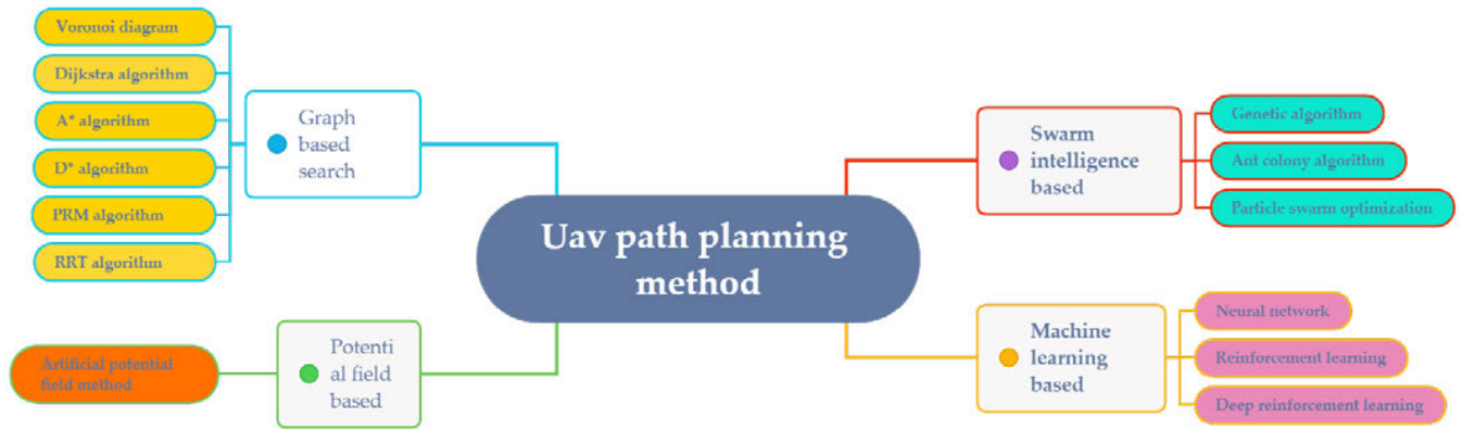
FIGURE 15. Classification chart of UAV path planning methods.
