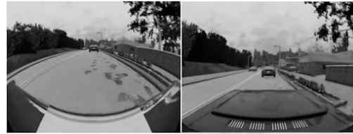
Fig. 15. Illustration of near and far-field front camera images forming an asymmetric stereo pair.
