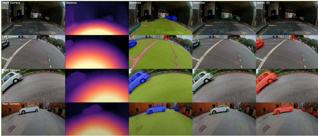
Fig. 14. Qualitative results of raw fisheye images from the OmniDet framework on the WoodScape dataset [2]. The 1 st column indicates the input images from Front, Left, Right and Rear cameras, 2 nd column indicate distance estimates, 3 rd column semantic segmentation maps, 4 th indicate generalized object detection representations and 5 th indicate the motion segmentation. For more qualitative results at a higher resolution, check this video: https://youtu.be/xsJz5OfPes .
