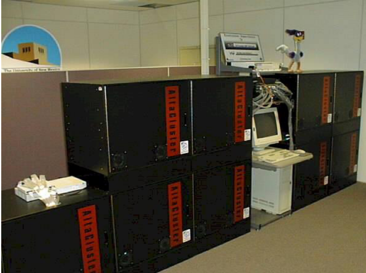
Figure 3: Linux prototype on lower-left, and Roadrunner (right). A Myricom dual 8-port SAN Myrinet switch sits on top of the left-most cabinet of the prototype, and four octal 8-port SAN Myrinet switches (not visible) connect Roadrunner. Above Roadrunner's console is a 72-port Foundry Fast Ethernet switch with Gigabit uplinks to the vBNS and Internet. (Image credit: Courtesy of the author.)
