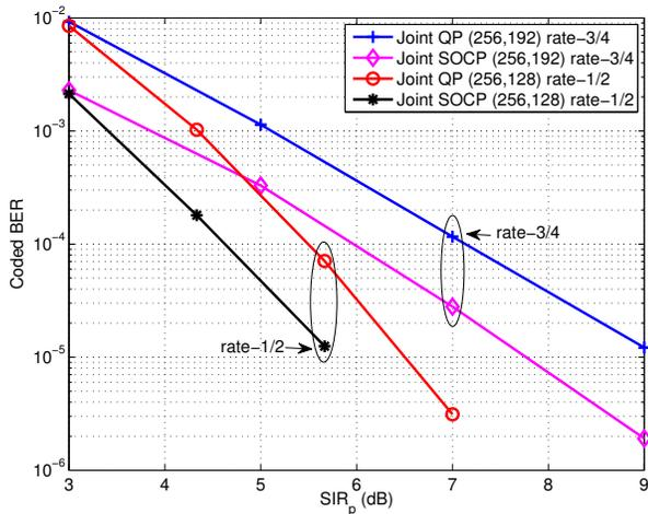
Fig. 6: BER comparisons with different code rates: (256,192) rate-3/4 versus (256,128) rate-1/2. 4-QAM.  $N_r = 32$ . Three users' seeds = (568,193,625). DL factor  $\gamma = 200\sigma_n^2$ . regularization parameter  $\alpha = 75$ . Chance constraints  $p = 0.95$ . Channel power gains = (1,  $I_p$ , 0.7).  $SIR_p \triangleq 10 \log_{10}(S/I_p)$ .
