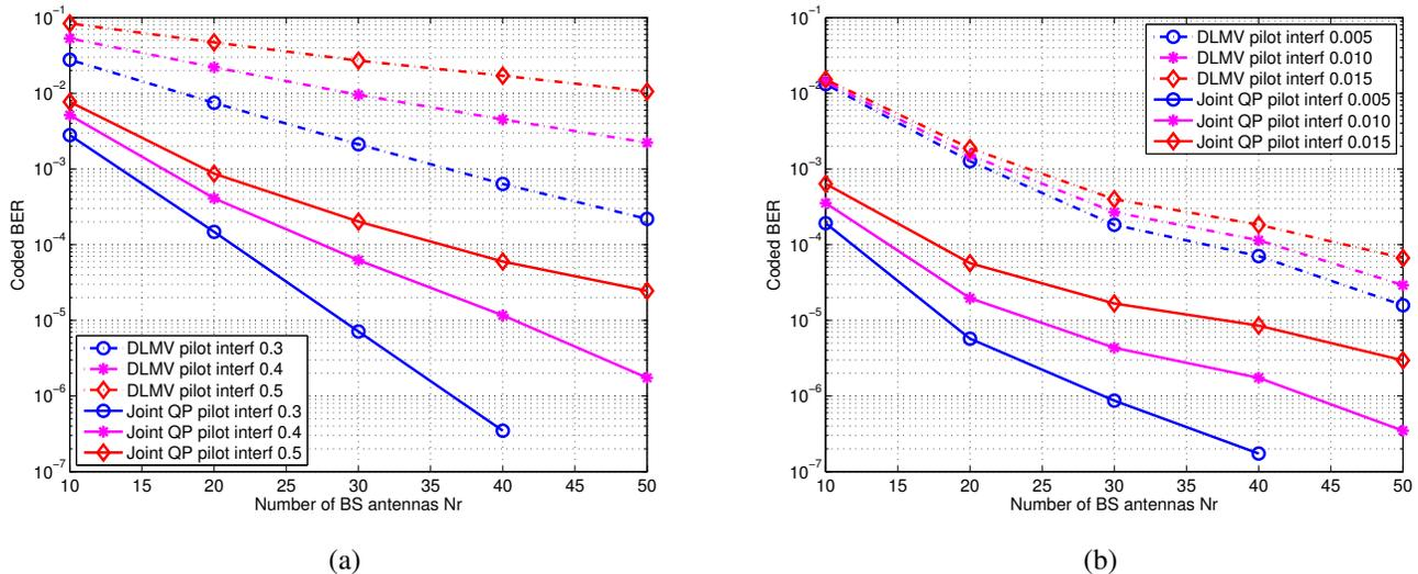
Fig. 5: BER versus number of BS antennas  $N_r$ : DLMV receiver and joint QP receiver. LDPC code (256,192). Three users' seeds = (568,193,625). (a) 4-QAM. SNR = 10 dB. Channel power gains =  $(1, I_p, 0.8)$  with pilot interference  $I_p = 0.3, 0.4$  and  $0.5$ . (b) 16-QAM. SNR = 15 dB. Channel power gains =  $(1, I_p, 0.6)$  with pilot interference  $I_p = 0.005, 0.010$  and  $0.015$ .
