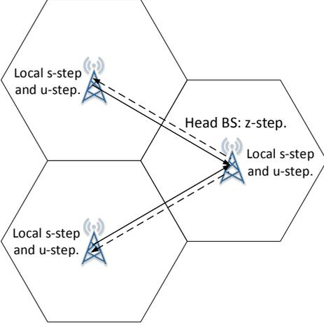
Fig. 2: ADMM process in an MC-MU-MIMO system: solid lines represent the flow direction of  $s$  and  $u$ ; dashed lines denote the flow direction of  $z$ .
