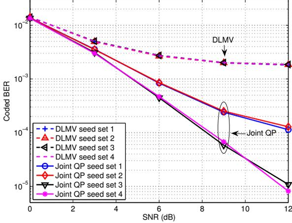
Fig. 3: Demonstration of code diversity effect: DLMV receiver versus joint QP receiver. 4-QAM.  $N_r = 32$ . LDPC code (256,192). DL factor  $\gamma = 200\sigma_n^2$  and regularization parameter  $\alpha = 75$ . Three users with channel power gains = (1, 0.3, 0.7). Seed set 1 = (568,568,568), set 2 = (568,568,625), set 3 = (568,193,568) and set 4 = (568,193,625).
