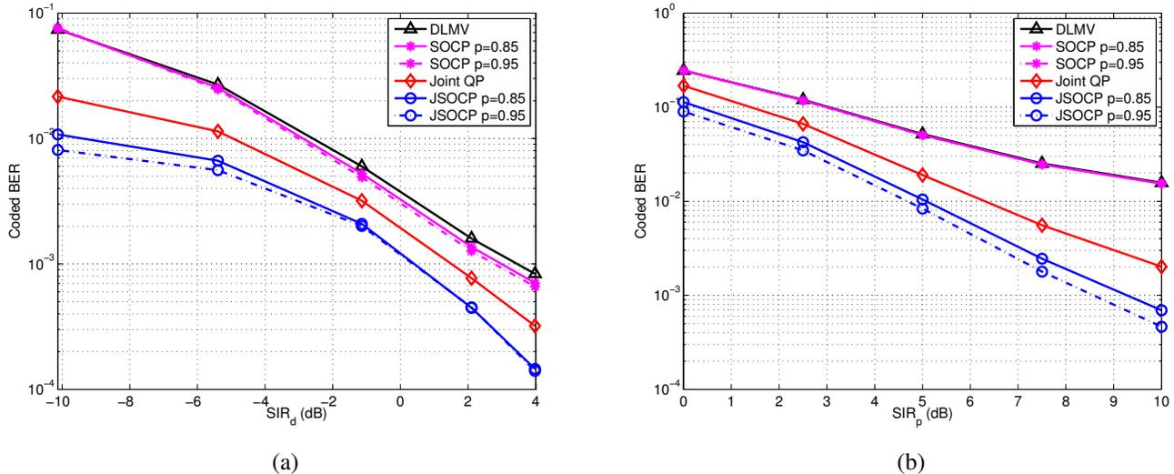
Fig. 4: BER versus data payload and pilot interference. 4-QAM.  $N_r = 32$ . SNR = 5dB. LDPC code (256,192). DL factor  $\gamma = 200\sigma_n^2$  and regularization  $\alpha = 75$ . (a) Fix  $I_p = 0.3$  and vary  $I_d$ . (b) Fix  $I_d = 0.7$  and vary  $I_p$ .
