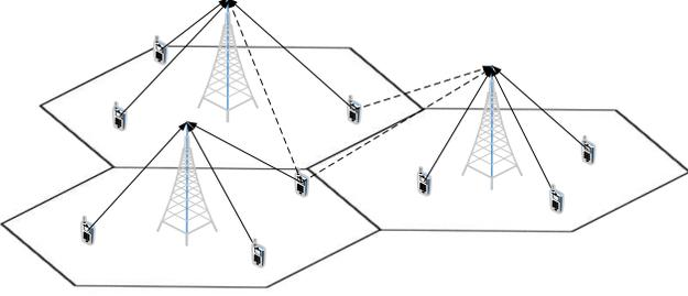
Fig. 1: Uplink transmissions in an MC-MU-MIMO system: solid lines denote intended signals and dashed lines represent interference signals.
