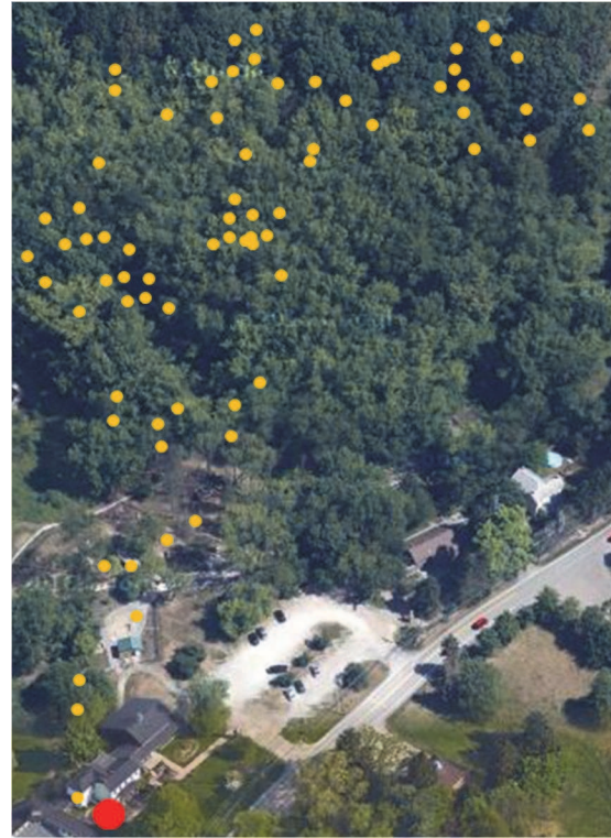
FIGURE 5. WSN testbed, sink locates at the red spot in the cabin house.
