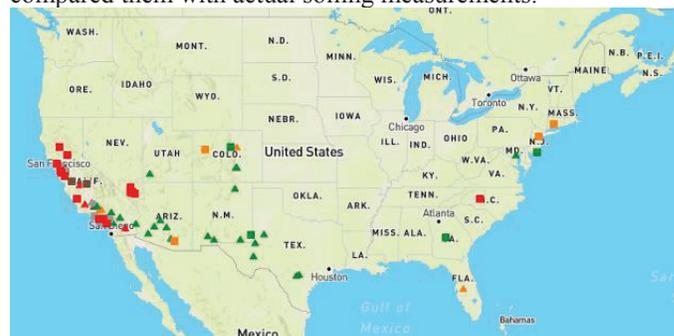
Fig. 1. Screenshot of the soiling map published in October 2017 on [www.nrel.gov/pv/soiling.html](http://www.nrel.gov/pv/soiling.html) [9]. Triangular markers (▲) are soiling stations; squared markers (■) are PV installations. The markers are color-coded according to the severity of soiling.
