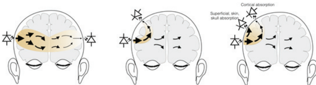
Figure 4: Different NIRS operation modes: Trans-illumination, reflectance and differential reflectance (redrawn after [77], [78]).
