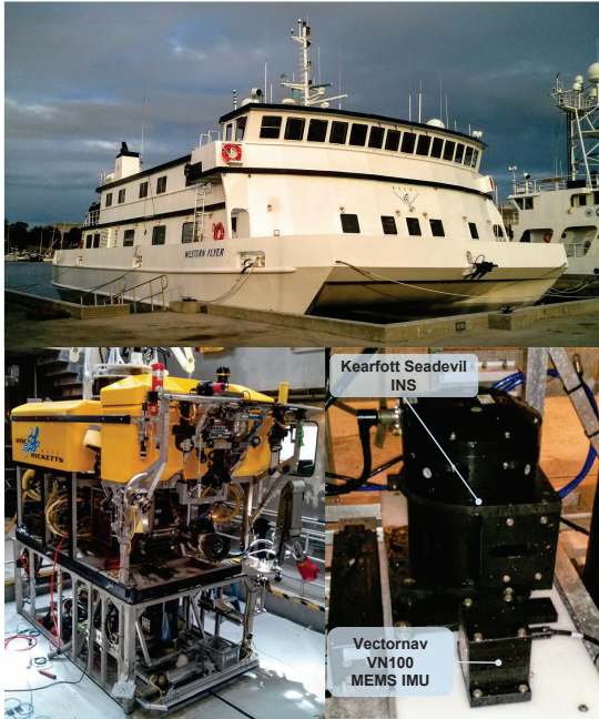
Fig. 10. MBARI R/V Western Flyer , ROV Doc Ricketts and detail of the sensors used in the field experimental evaluation
