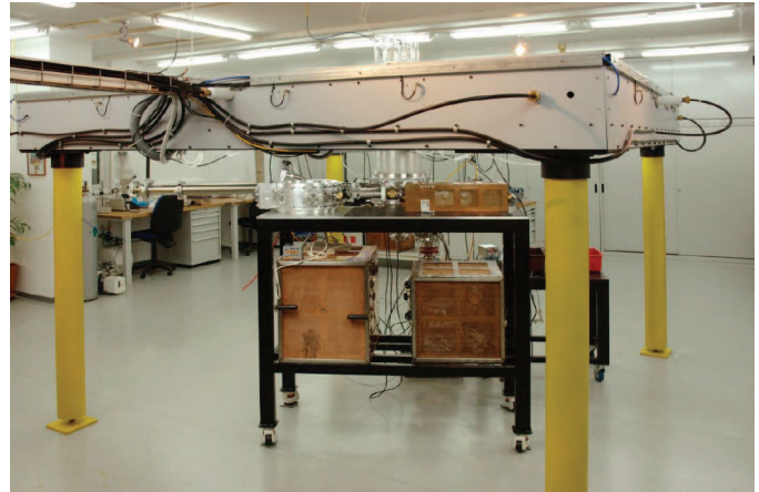
Fig. 29. Photograph of the 500-kA, 500-ns LTD at the Weizmann Institute of Science in Israel.
