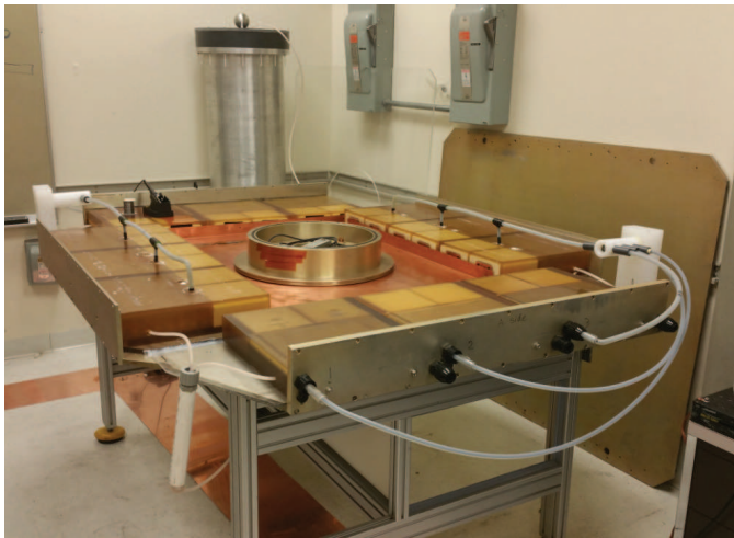
Fig. 32. Photograph of the 200-kA, 60-ns Lobo LTD at the University of New Mexico in Albuquerque.
