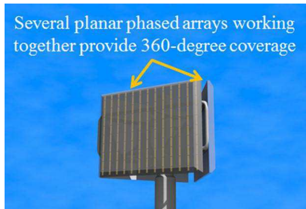
Fig. 2. Depiction of an 'ideal' base station utilizing optically-upconverted phased arrays with analog beam forming for spatial channelization.
